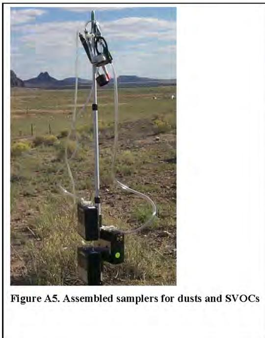
**Figure A5. Assembled samplers for dusts and SVOCs**
