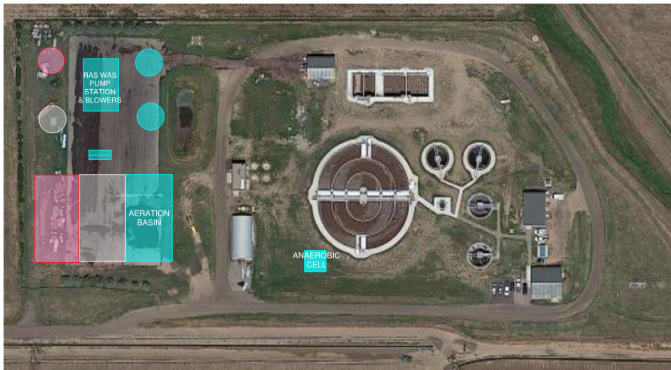
Figure 2-5. Conventional Activated Sludge with Stepfeed Expansion Option
